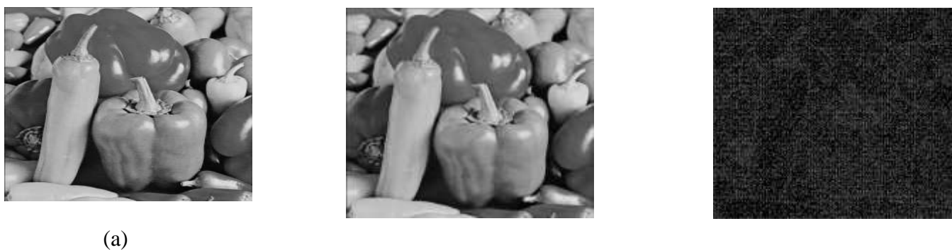
Figure 9: The results of eight-sided side match using sample arrangement as in Figure 1 with Peppers image (a) original-image, (b) stego-image and (c) difference image.
