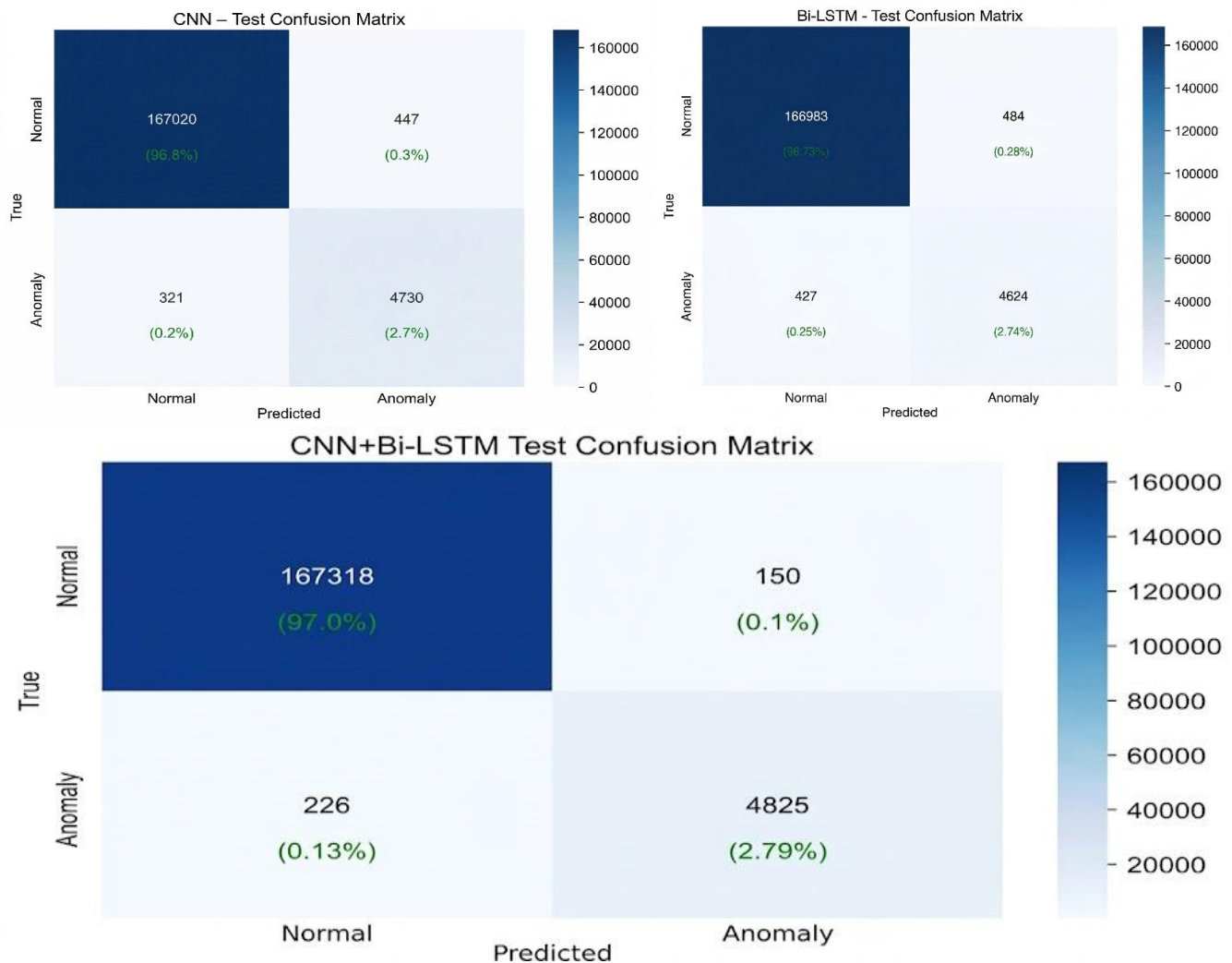
Figure 5: The confusion matrix illustrating the experimental results of each model on the HDFS dataset.
