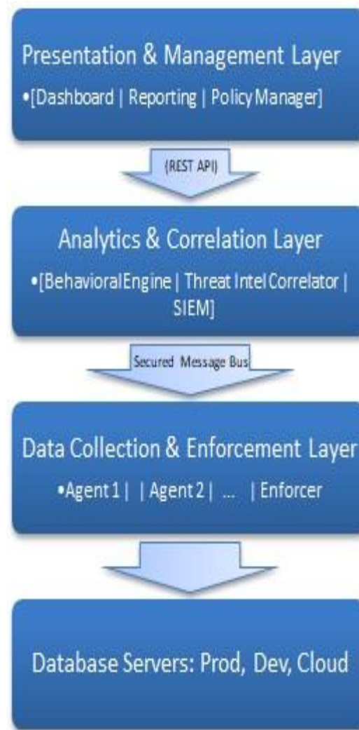
Fig. 1 - DBCS High-Level Architecture.
