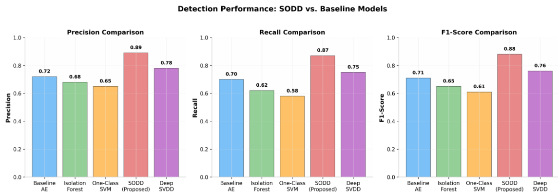
Figure 5. Detection performance comparison across Precision, Recall, and F1-Score metrics. SODD (proposed) demonstrates consistent superiority over baseline methods including standard Autoencoder, Isolation Forest, One-Class SVM, and Deep SVDD.
