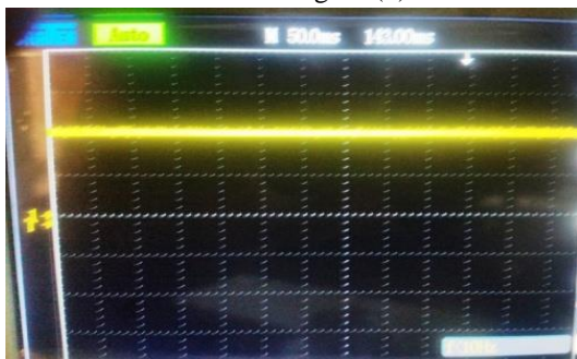
Figure 5. The Output of Dust Sensor without Dust
