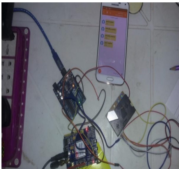
Figure 12. The implemented SIM900 Board
