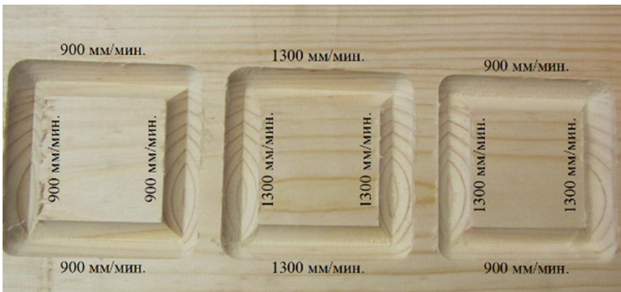
Figure 4 – Result of pine wood surface milling (supply rate along the milling contour sides is indicated in mm/min)
