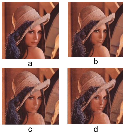
Figure 4: Lena a) Original b) RGB & KMCG c) YCbCr & KMCG d) HSV & KMCG
